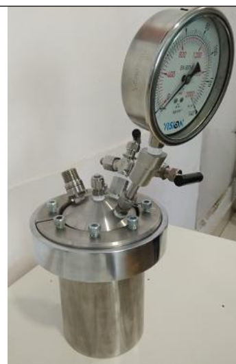
1000 ml Vessel removable head, gauge, rupture disk and Valves
